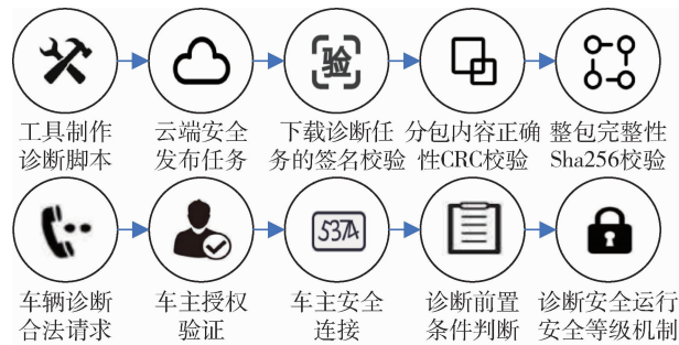
图4 诊断任务脚本及诊断数据安全流程示意图 Fig. 4 Schematic Diagram of Diagnostic Task Script and Data Security Process
